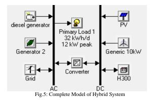
Converter converts the DC outputs of the PV system and battery into AC. The loads are considered to be AC loads.
