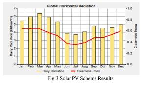
The solar radiation for each month was obtained where it was found that the maximum solar radiation was found for the month of February and March with daily radiation of 6.390kWh/m<sup>2</sup>/day whereas the minimum radiation was found for the month of July with daily radiation 3.710kWh/m<sup>2</sup>/day. The average radiation throughout the year was 4.971kWh/m<sup>2</sup>/day.
